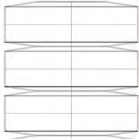
Figure 7: V-shaped connectors create springy tension in the folds.
