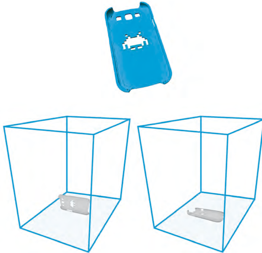
Figure 8. Left: A phone case to be printed. Middle: The suggested orientation for minimizing warpage when there is a low probability of bowing. Right: An alternative orientation that minimizes the bowing effect while still being a good option for reducing warpage
