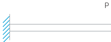
Figure 10. Cantilever beam with a point-applied end load
