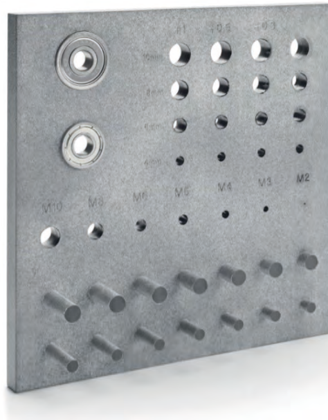
Figure 3: Bearings inserted into an HP MJF part
